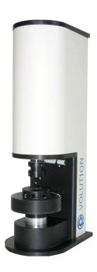
Flowability of Powder under Load: measurement in ring shear cells is used to determine flowability data according to the Mohr-Coulomb model. The resulting values can be used for designing silos or to predict powder flow under load.
