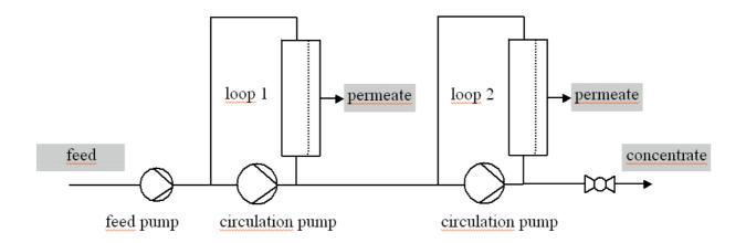
The following formulae are resulting from material balance calculated for a continuous membrane process with one loop.
